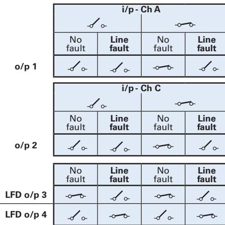
**Mode 12:** 3 ch with common LFD output
