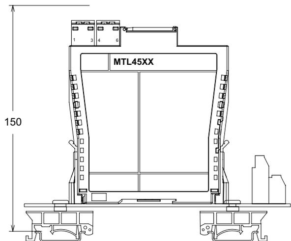
**Figure 4.1: Standard backplanes with dimensions**
