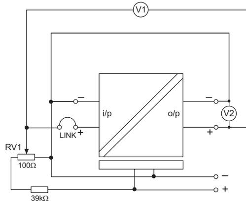
Note: V1 should be capable of measurement to within  $1\mu\text{V}$ .
