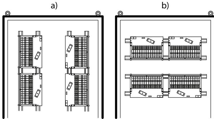
**Figure 5.2: Backplane orientations when mounted in cabinets**
