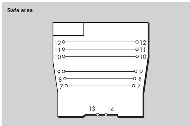
Note: Must not be used with signals >50V or >0.25A
