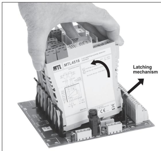
Figure 5.5: Removing a module from a backplane
