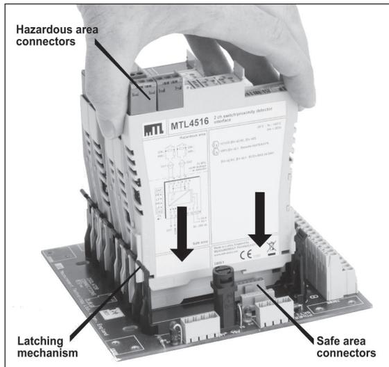
Figure 5.4: Mounting a module onto a backplane
