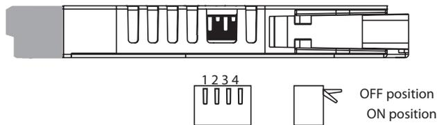
The switch setting options are always indicated on the side label of the module, but the user may also consult the individual module information in Section 6 of this manual for details.
