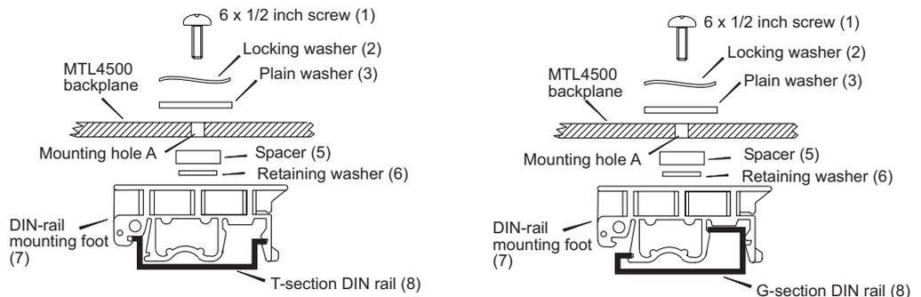
**Figure 4.3: Mounting a backplane onto 'T' or 'G' section DIN rail**
