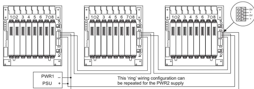
**Figure 4.11:** "Ring main" wiring for DC power
