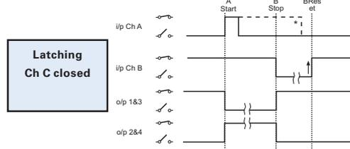
\* i/p Ch A can be open or closed when i/p Ch B opens to stop latch
