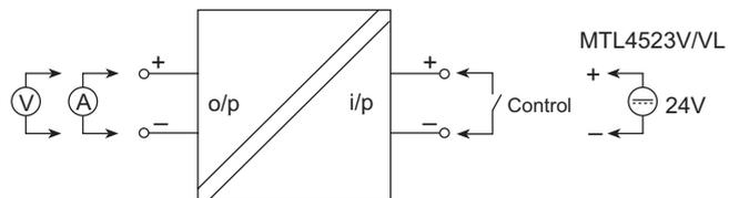
1. Connect a voltmeter between the + & - output terminals of the module, observing polarity
