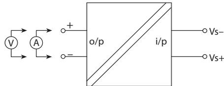
1. Connect a voltmeter between the + & - output terminals of the module, observing polarity.
